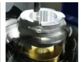
Vibration caused by imbalance of the jig or workpiece during C-axis rotation has been minimized, achieving stable rotation to prevent the decrease in machining accuracy.
