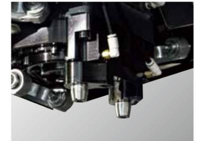
An original double plunger lock is used to secure turning tools, achieving excellent tool change repeatability.
